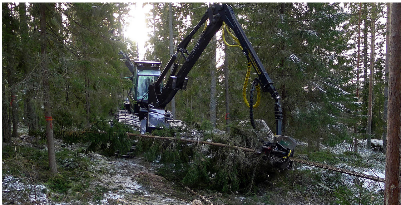
Figure 1. Trees are being cut and the stems are delimbed and cross-cut.
